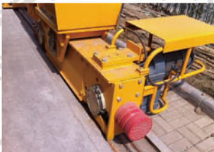
三合一电机柔性直驱 Impacted gearmotor
