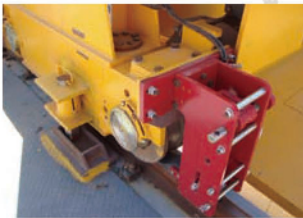
电动液压防风铁靴 Electro-Hydraulic storm braking wedge
